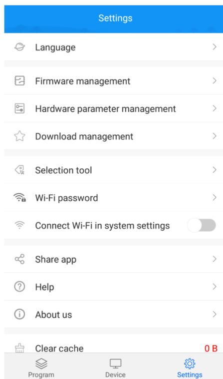
Among them, the firmware management and hardware parameter management are functions only for the LED single and double color W series; the selection tool is also made for the selection of LED control card.
