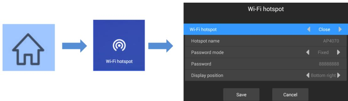
Press the menu key on the remote control, select Wi-Fi hotspot, and turn on Wi-Fi hotspot.
